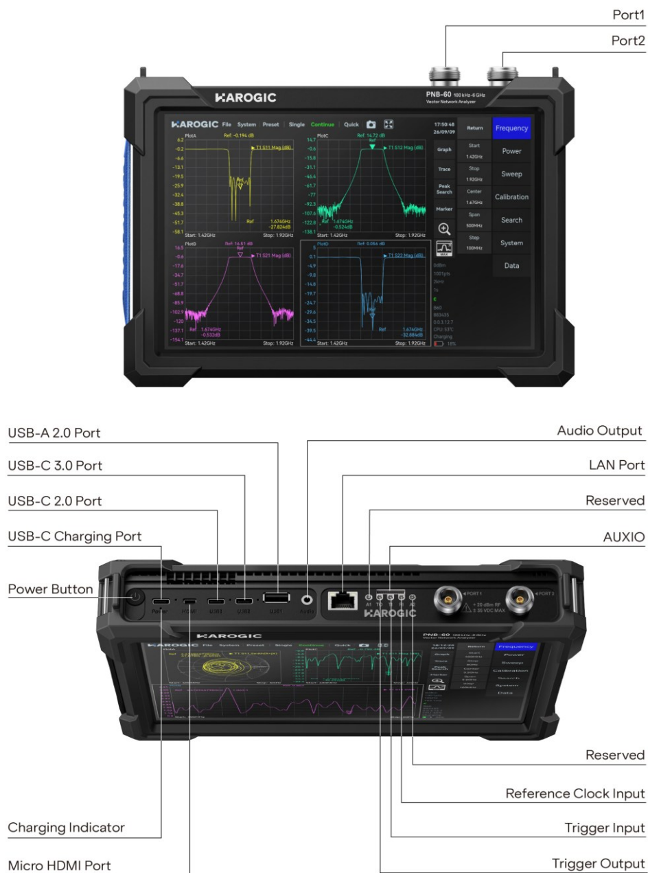
Figure 2 PNB Series Interface Description
