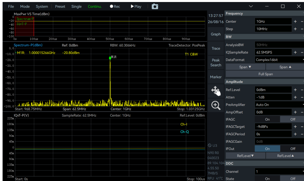
Figure 8-2 IQ Streaming Test Results Measured with the R1090 RF Receiver
