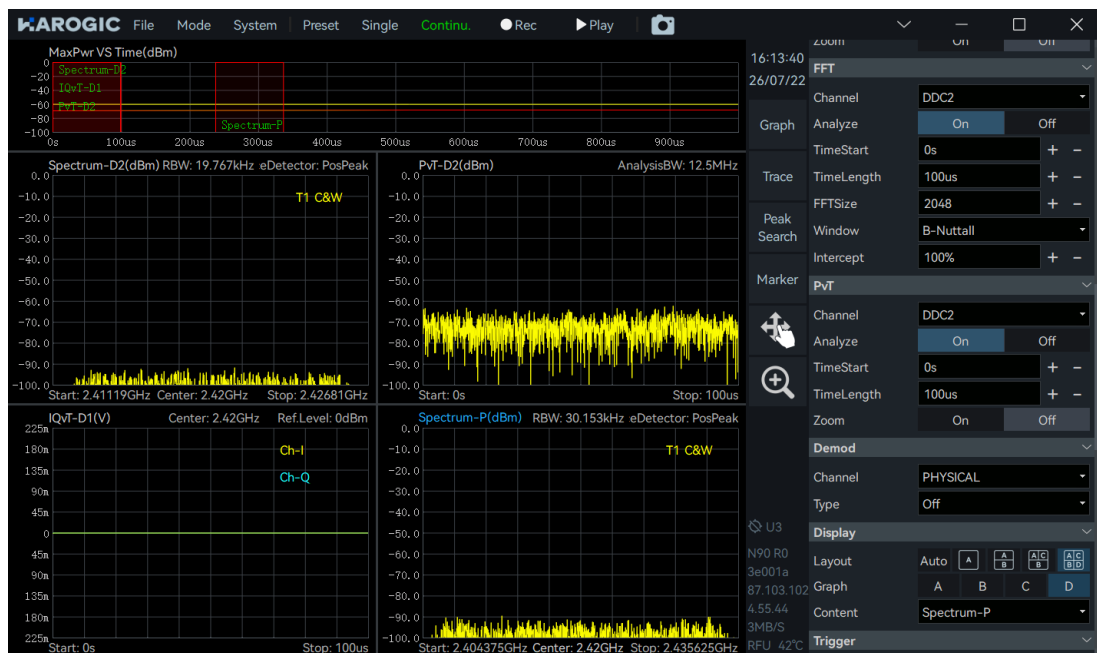
Figure 8-5 DDC Multi-Channel Target Sub-Band Analysis in Receiver IQ Streaming Mode
