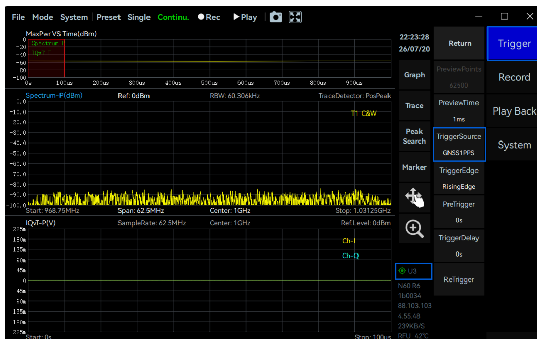
Figure 8 Triggered using GNSS 1 PPS
