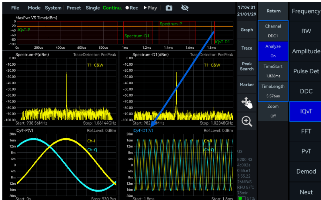
Figure 37 View the time-domain diagram of the IQ subflow under DDC
