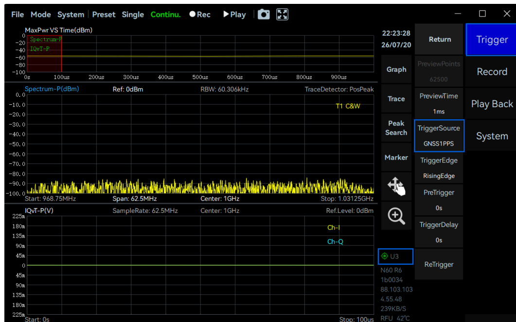
Figure 8 Triggered using GNSS 1 PPS
