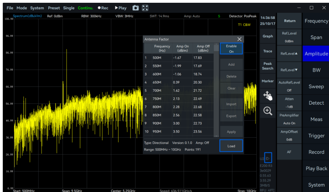
Figure 30 With HDA-100: automatic loading of antenna factors
