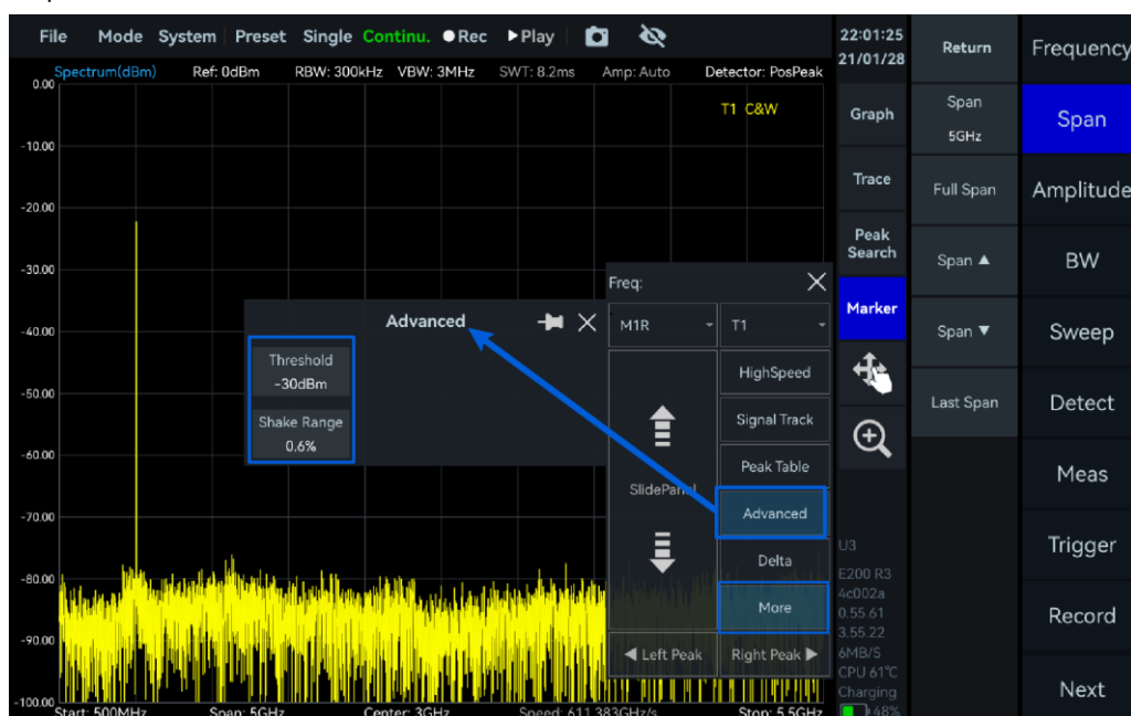
Figure 16 Set the Peak Threshold and Shake Range
