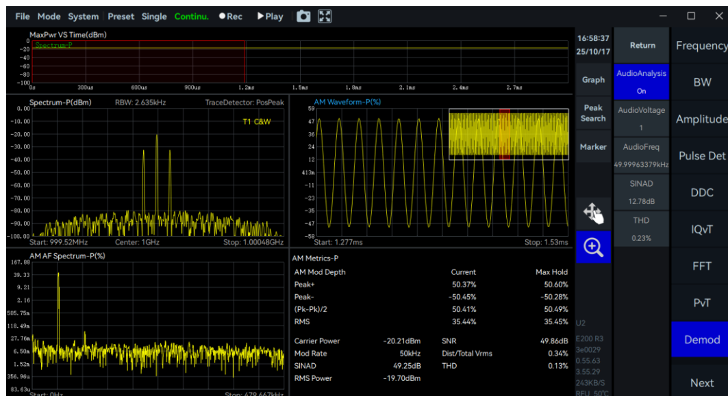
Figure 35 Audio analysis of AM demodulation
