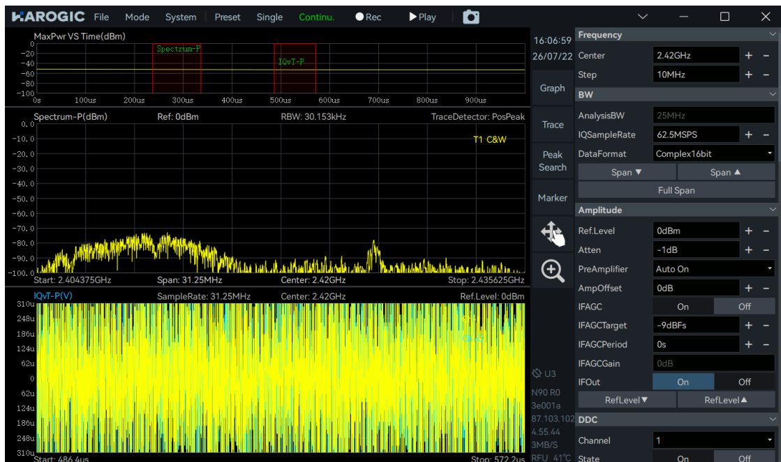
Figure 8-3 Spectrum and IQ Time-Domain Waveform in Receiver IQ Streaming Mode
