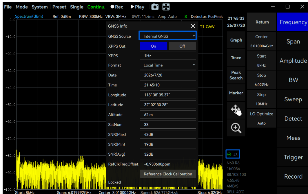
Figure 5 Use the internal GNSS source
