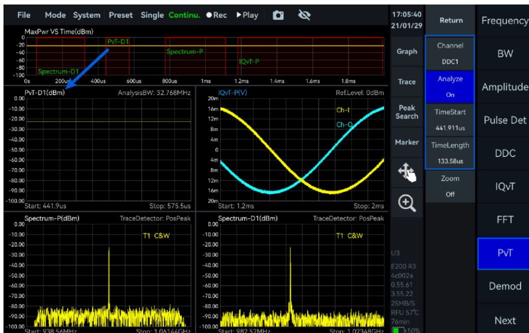
Figure 38 View the power-time graph of the IQ subflow under DDC
