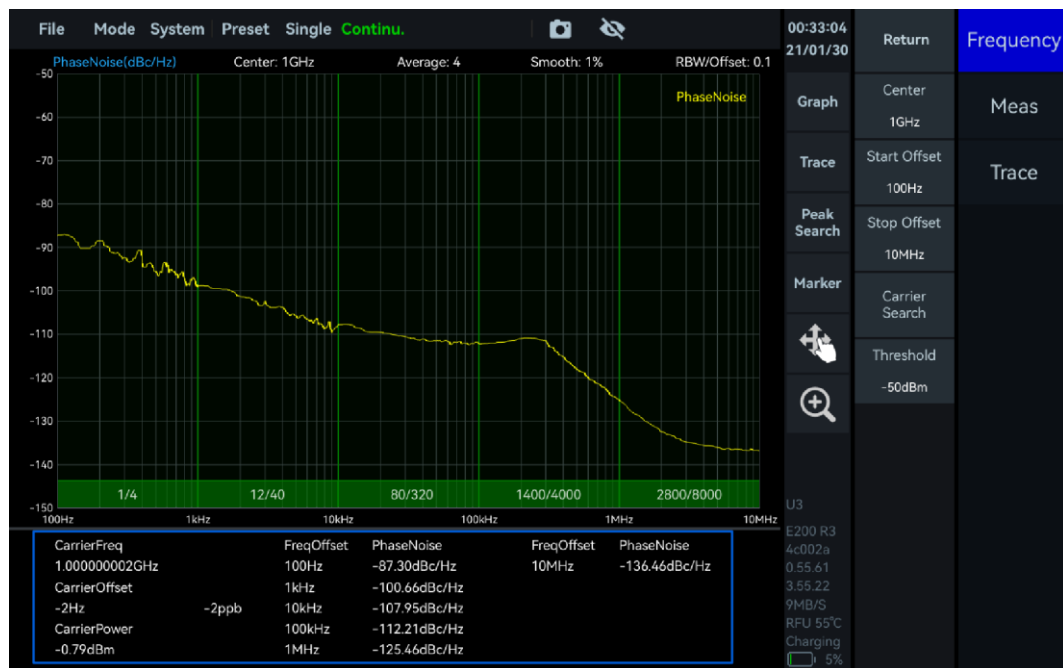
Figure 46 Result of Phase Noise Measurement
