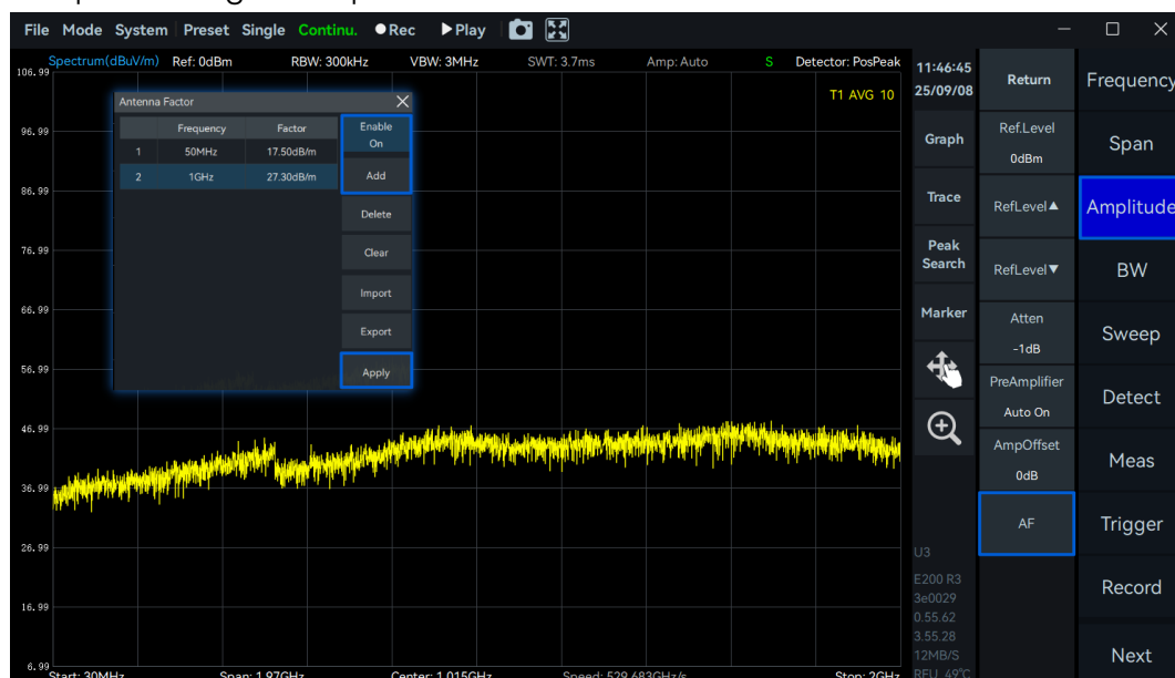
Figure 29 Antenna Factor Configuration Example
