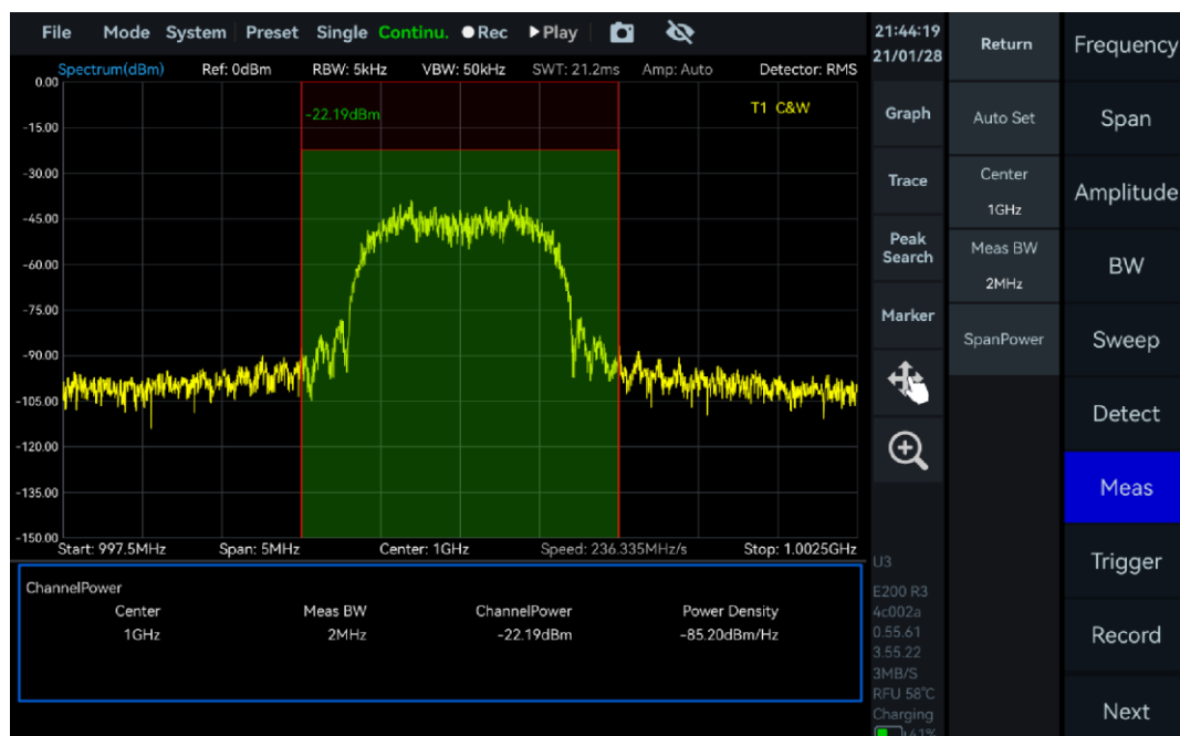
Figure 23 Measurement of ChannelPower
