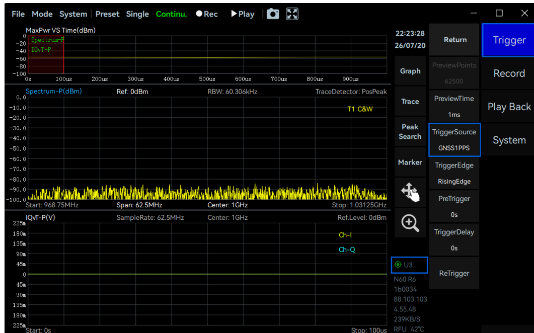
Figure 8 Triggered using GNSS 1 PPS
