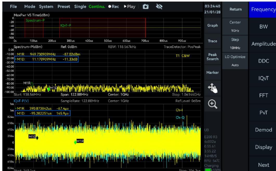
Figure 15 Enable Delta Marker
