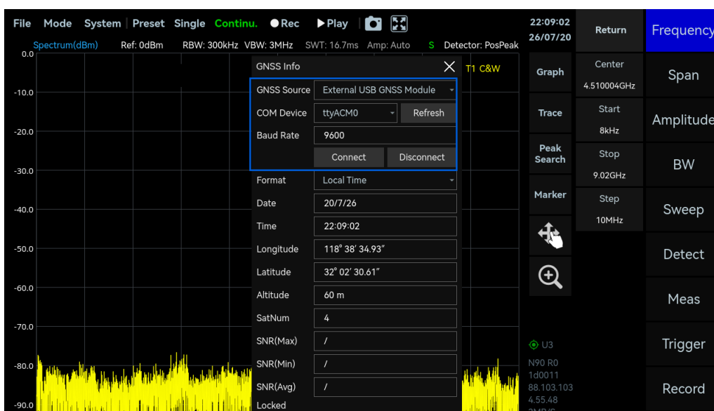
figure 7 Connect the external GNSS module
