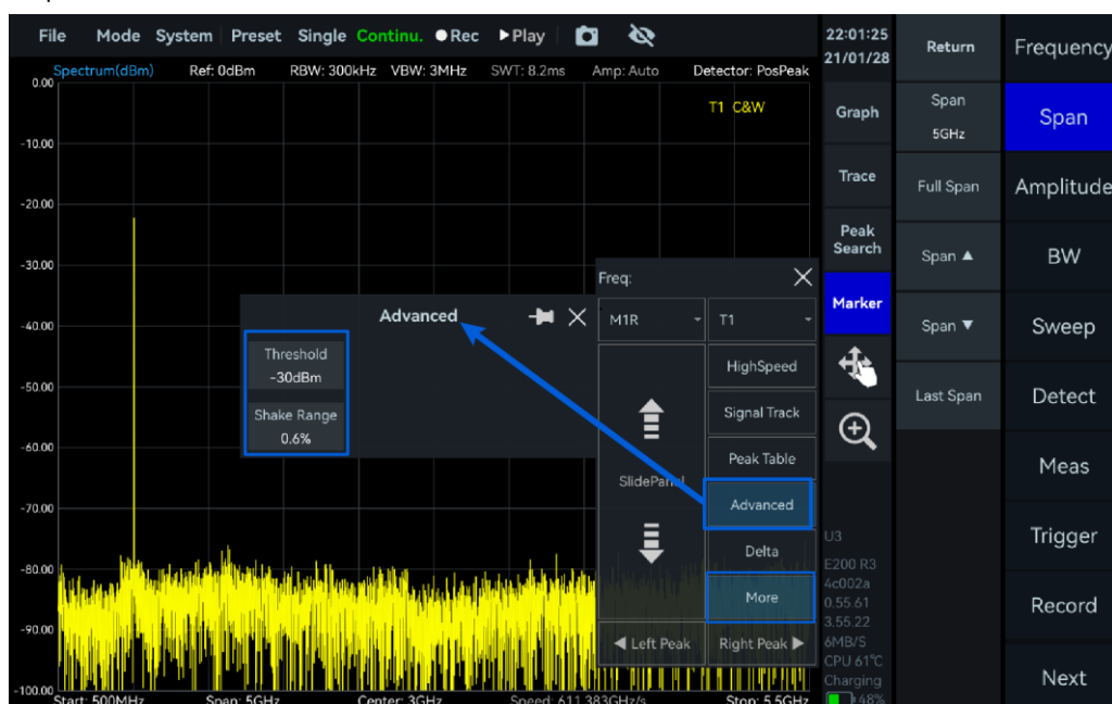
Figure 16 Set the Peak Threshold and Shake Range
