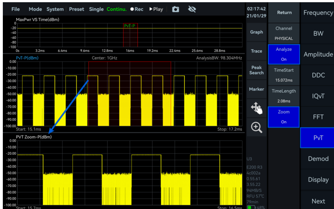
Figure 33 IQ Power-Time Plot and Zoom
