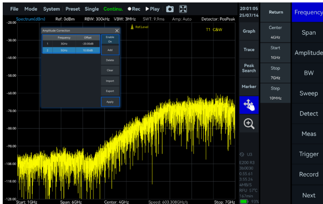
Figure 20 Amplitude correction application
