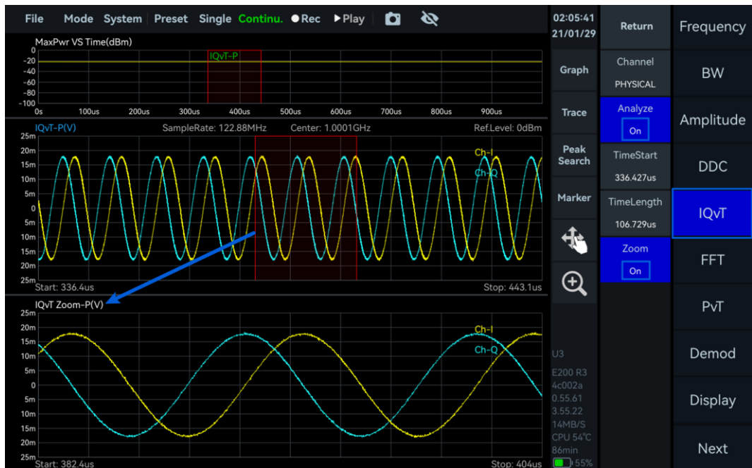
Figure 32 IQ Time-Domain Plot and Zoom
