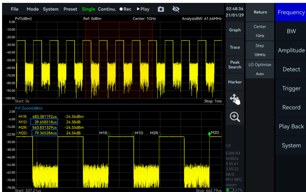
Figure 39 Pulse Signal Period and Width Measurement
