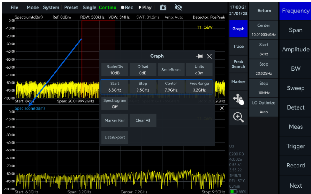
Figure 13 Spectrum zoom in SWP mode
