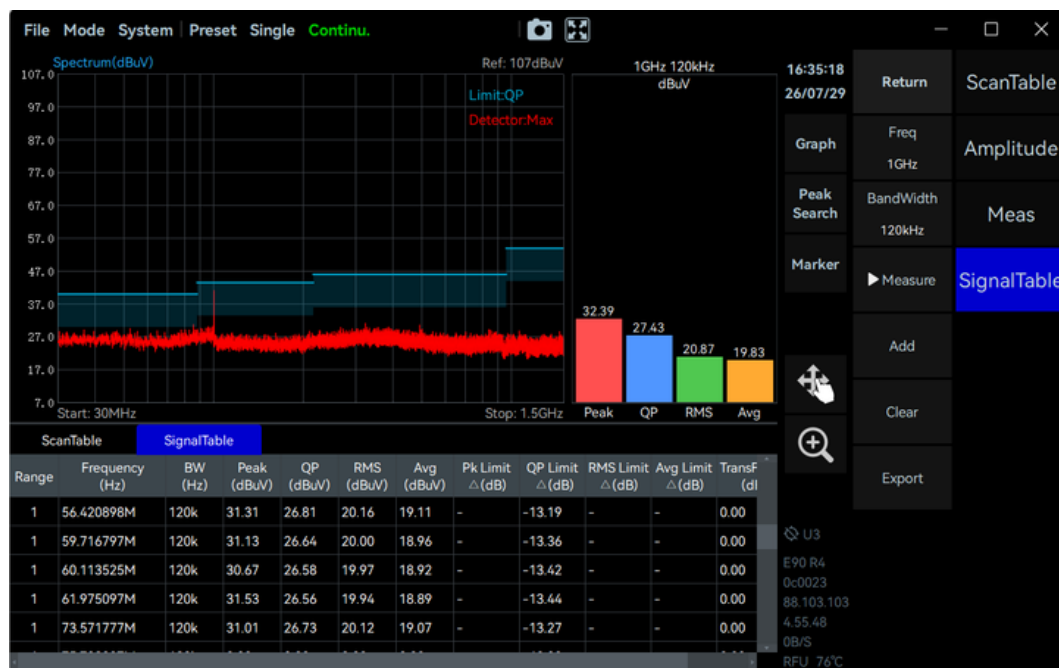
figure 53 EMC Measurement Diagram
