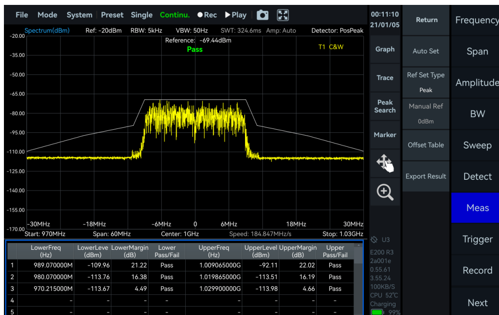
Figure 27 Measurement of SEM
