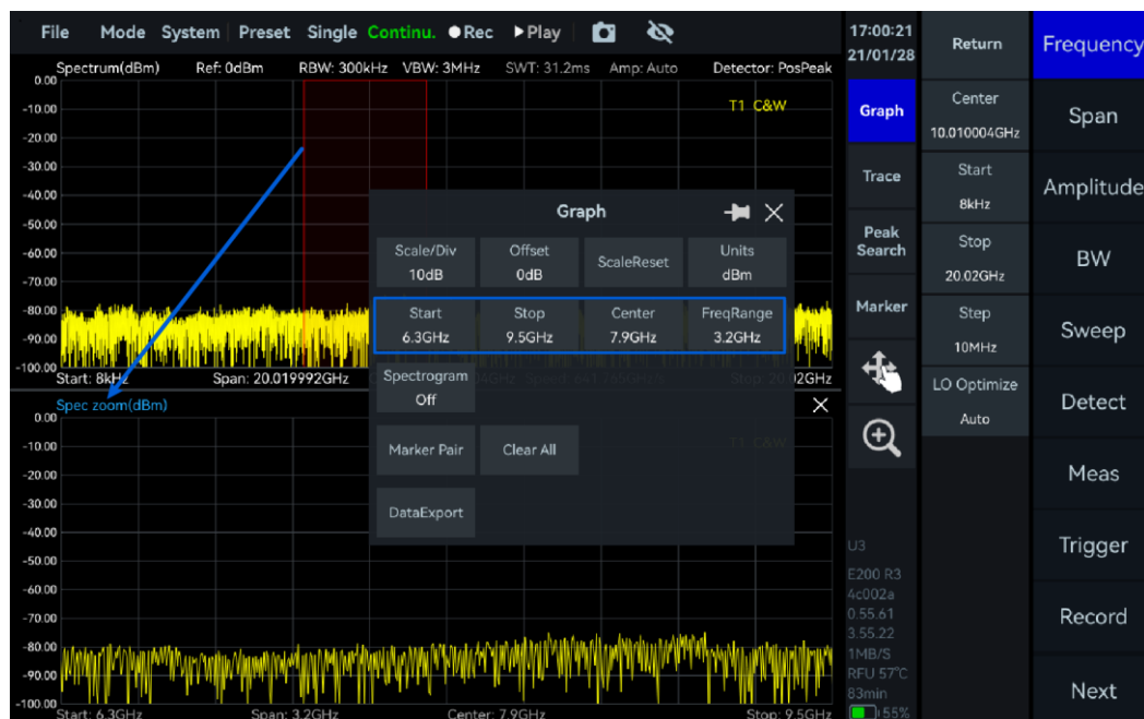
Figure 11 Spectrum zoom in SWP mode
