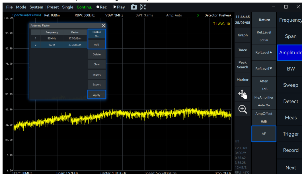
Figure 27 Antenna Factor Configuration Example
