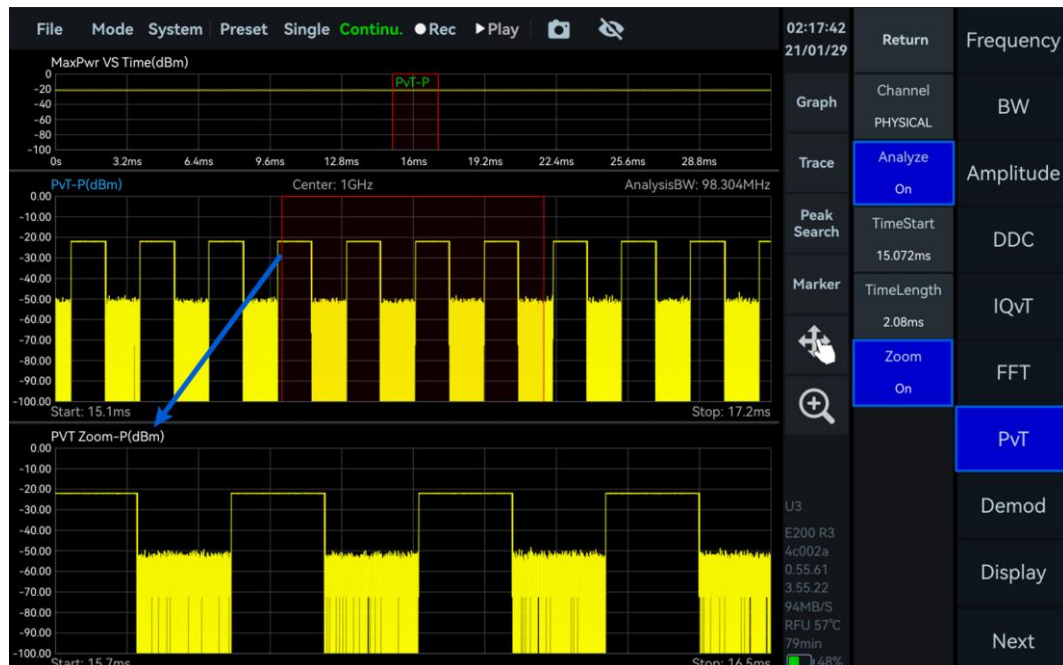
Figure 31 IQ Power-Time Plot and Zoom
