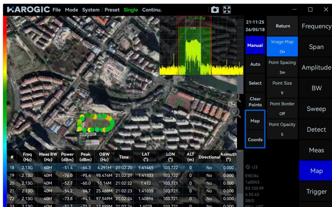
Figure 45 Heatmap Corresponding to Custom Image Map Mode
