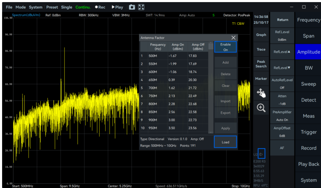
Figure 28 With HDA-100: automatic loading of antenna factors
