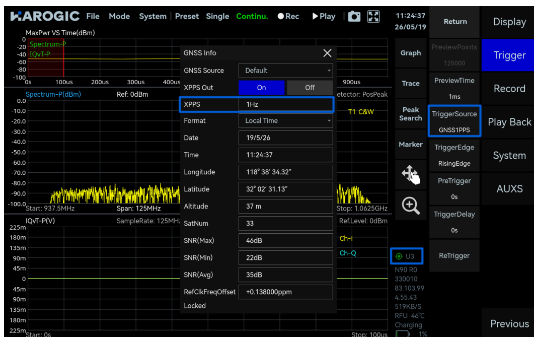
Figure 6 Triggered using GNSS 1 PPS
