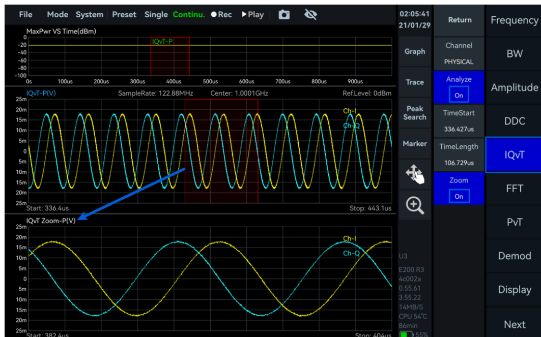
Figure 30 IQ Time-Domain Plot and Zoom
