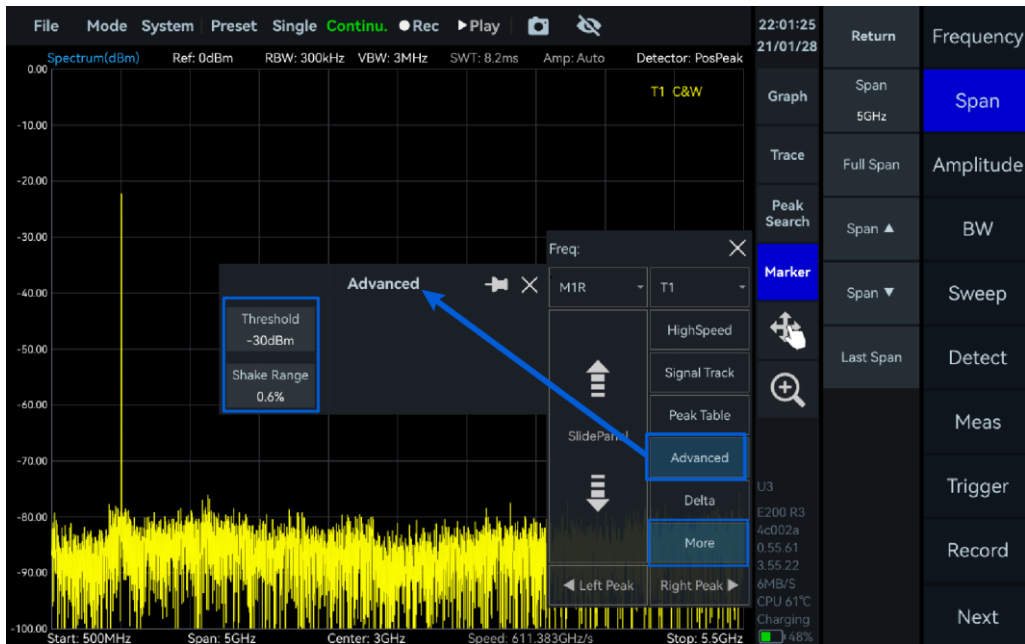
Figure 14 Set the Peak Threshold and Shake Range
