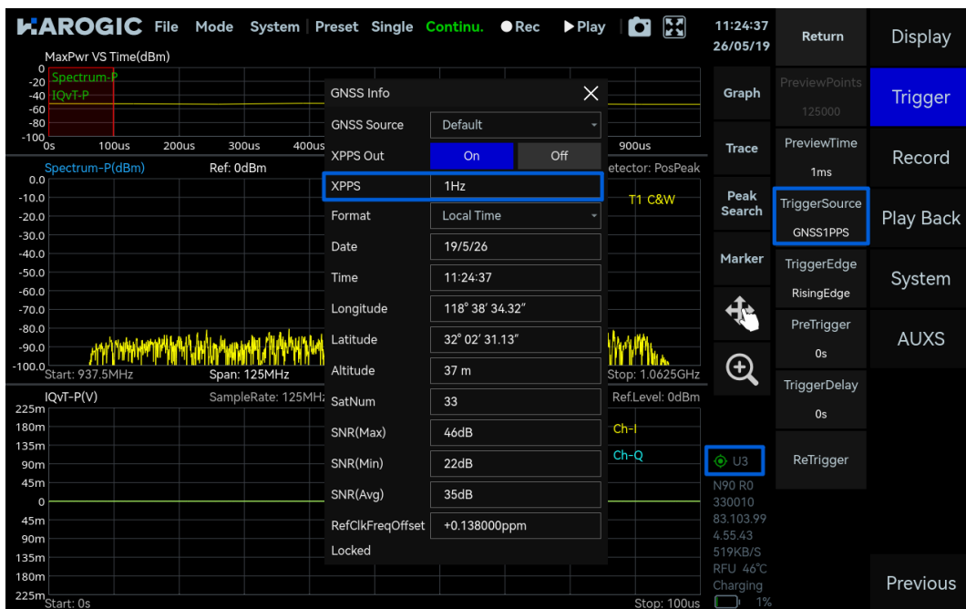
Figure 6 Triggered using GNSS 1 PPS
