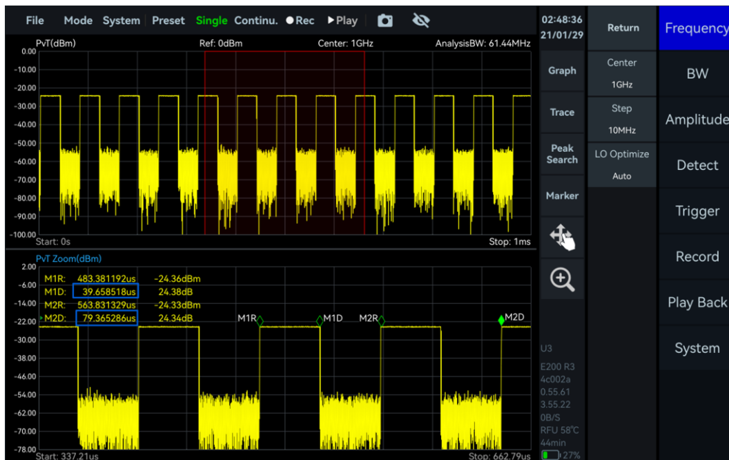
Figure 35 Pulse Signal Period and Width Measurement
