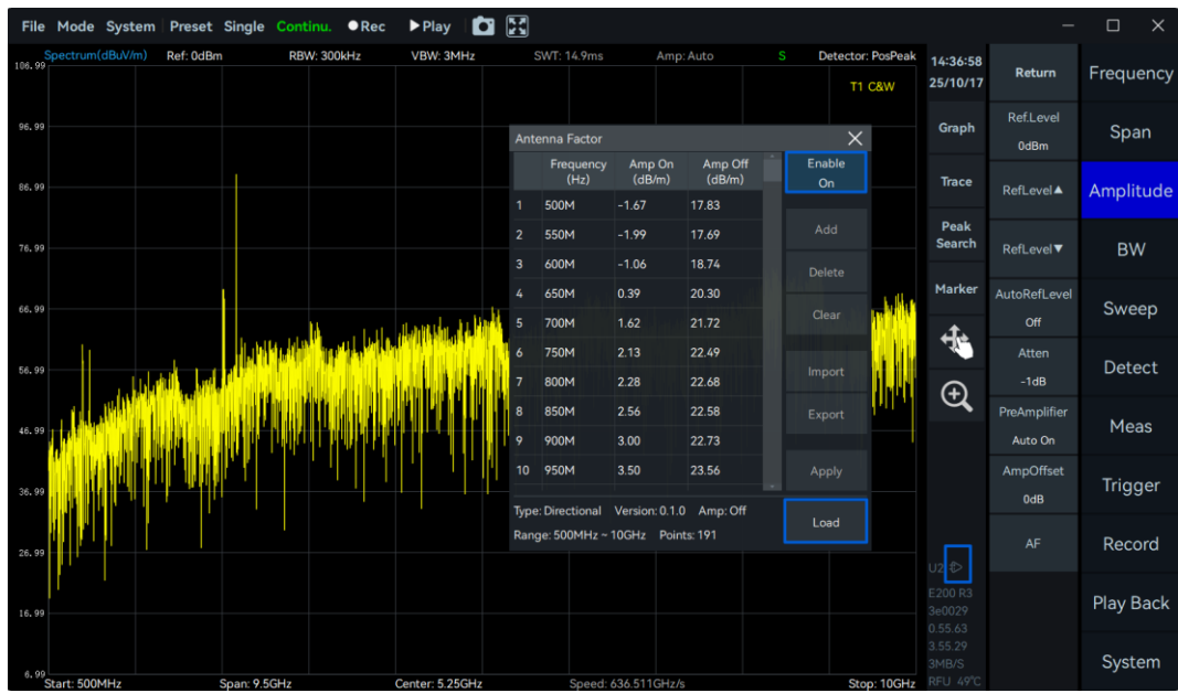
Figure 26 With HDA-100: automatic loading of antenna factors
