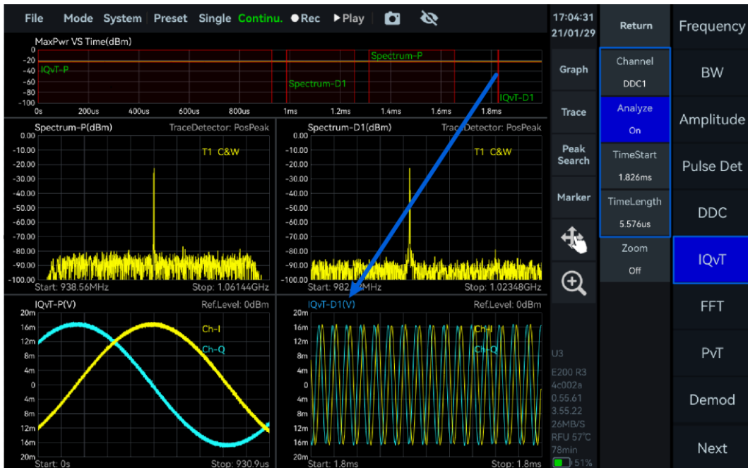
Figure 33 View the time-domain diagram of the IQ subflow under DDC
