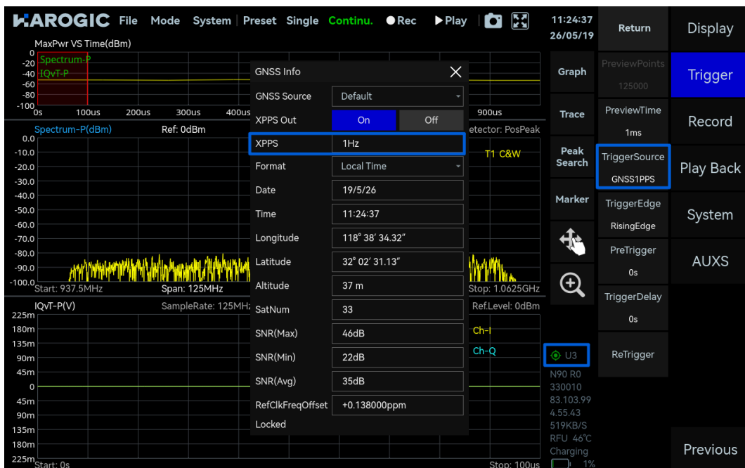
Figure 6 Triggered using GNSS 1 PPS
