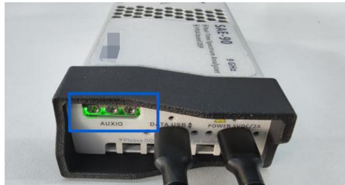
Figure 11 Indicator light of SAE and SAN-400 series instruments
