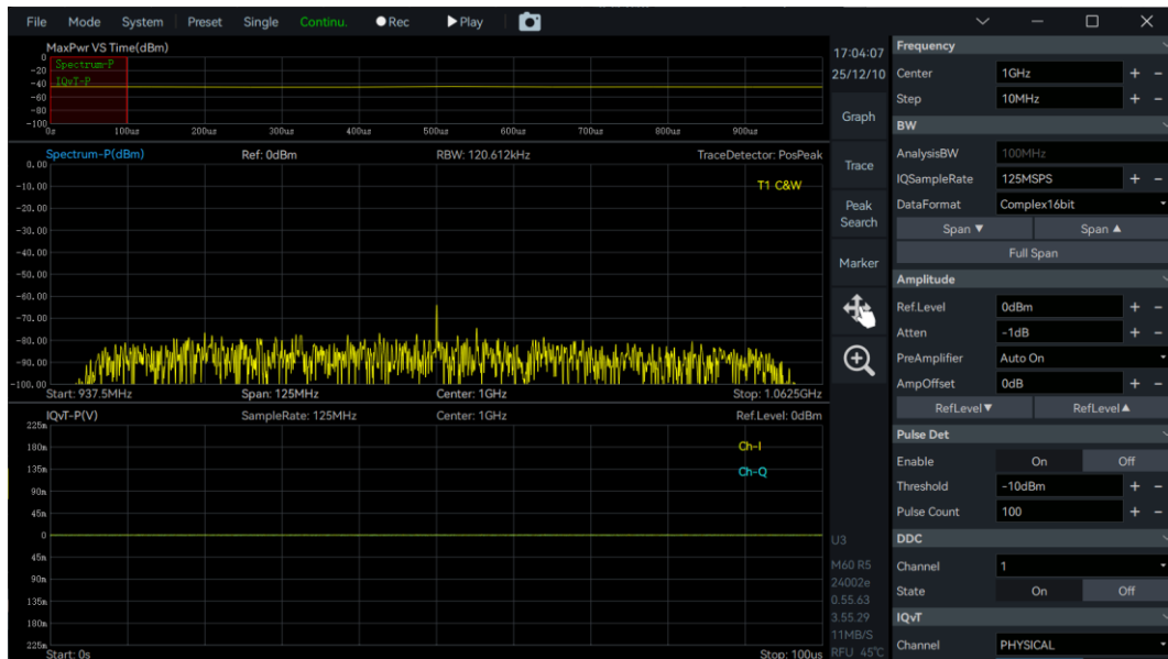
Figure 23 Observed signal power deviation phenomenon in IQ mode
