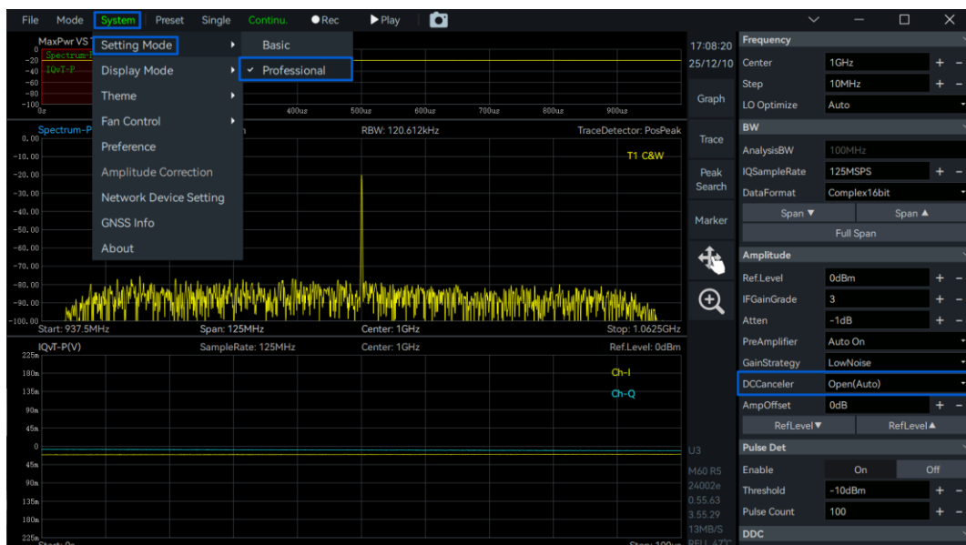
Figure 24 Enable High-Pass Filter Function in IQ Mode
