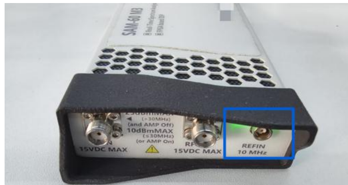
Figure 12 Indicator light of SAM and SAN series instruments
