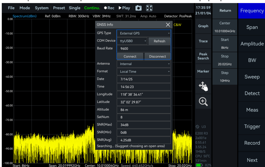
Figure 8 Connecting an external GNSS module
