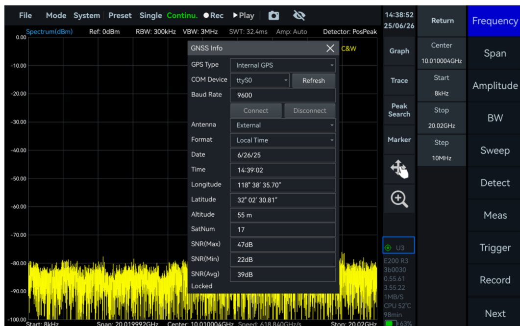
Figure 5 Locked GNSS external antenna
