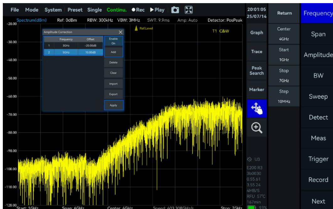
Figure 17 Amplitude correction application
