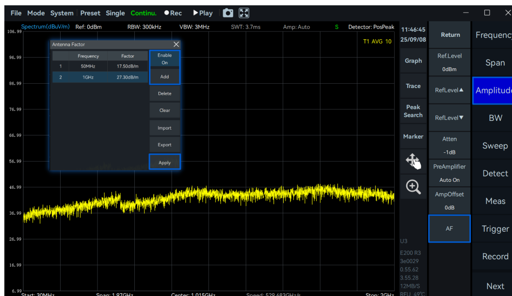
Figure 24 Antenna Factor Configuration Example
