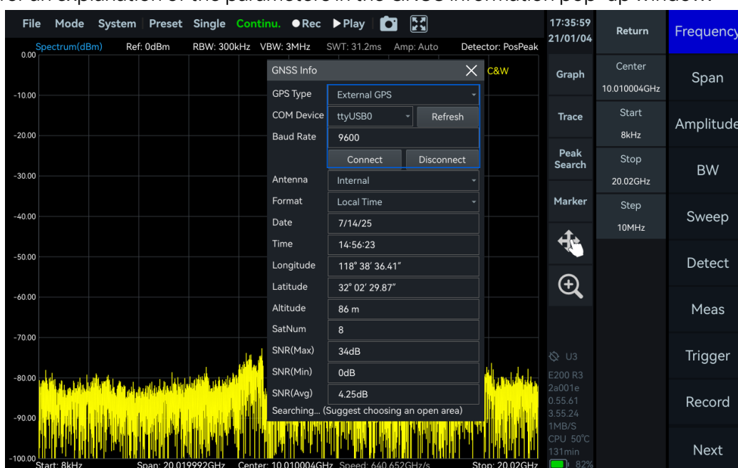
Figure 8 Connecting an external GNSS module
