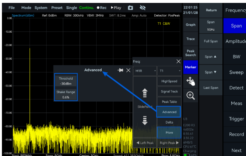
Figure 13 Set the Peak Threshold and Shake Range
