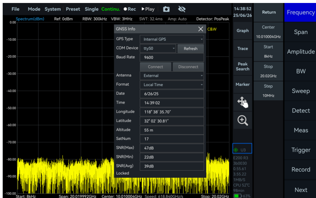
Figure 5 Locked GNSS external antenna
