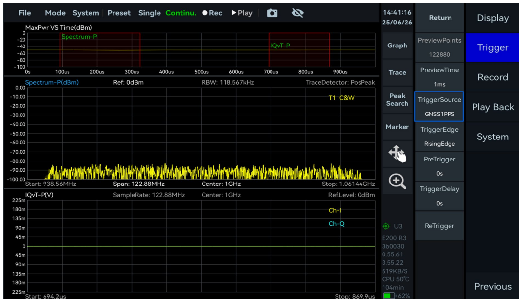
Figure 6 Triggered using GNSS 1 PPS
