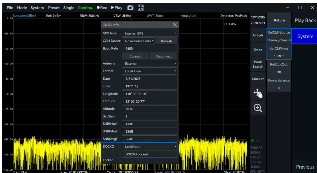
Figure 7 10MHz reference clock using high quality GNSS modules
