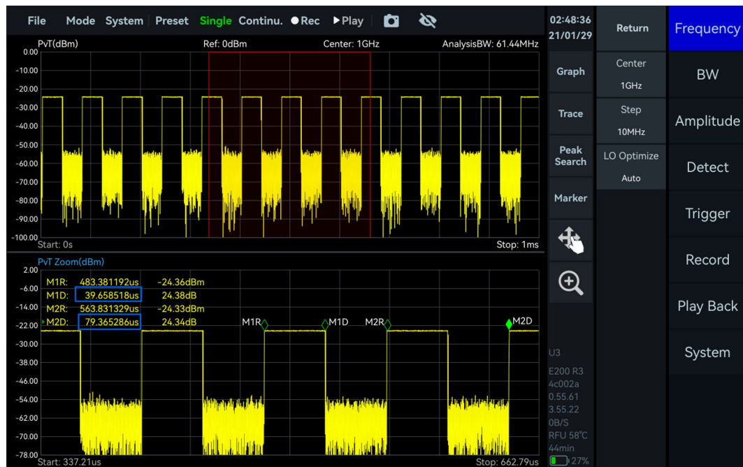
Figure 31 Pulse Signal Period and Width Measurement
