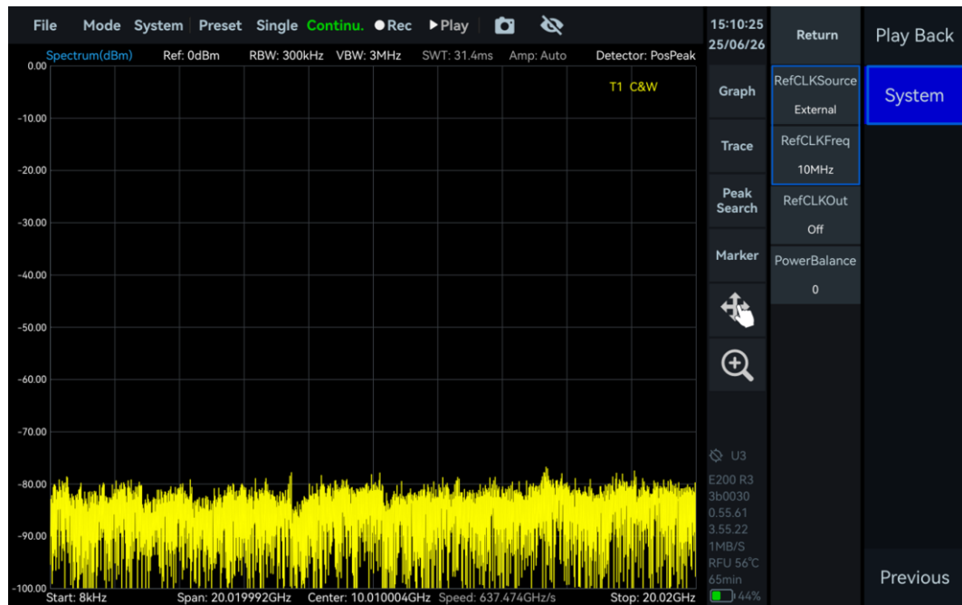
Figure 45 Use an external 10 MHz reference clock
