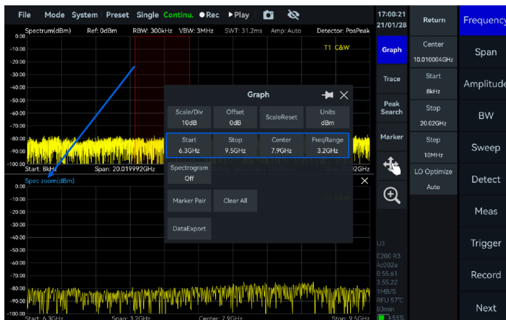
Figure 10 Spectrum amplification in SWP mode
