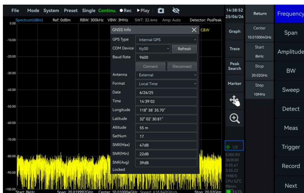
Figure 5 Locked GNSS external antenna
