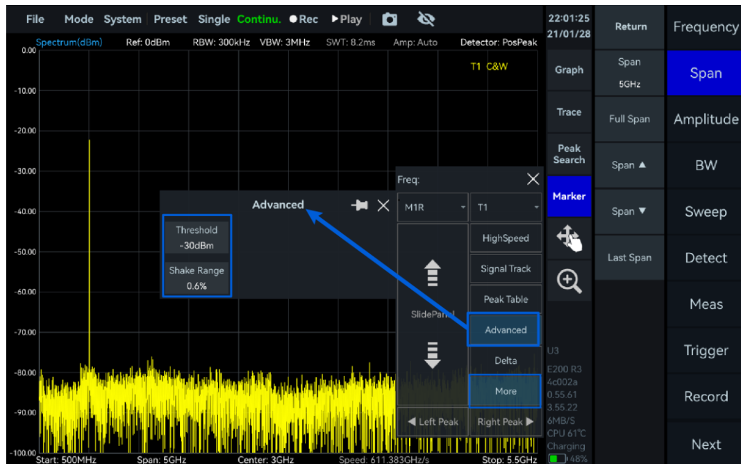
Figure 13 Set the Peak Threshold and Shake Range
