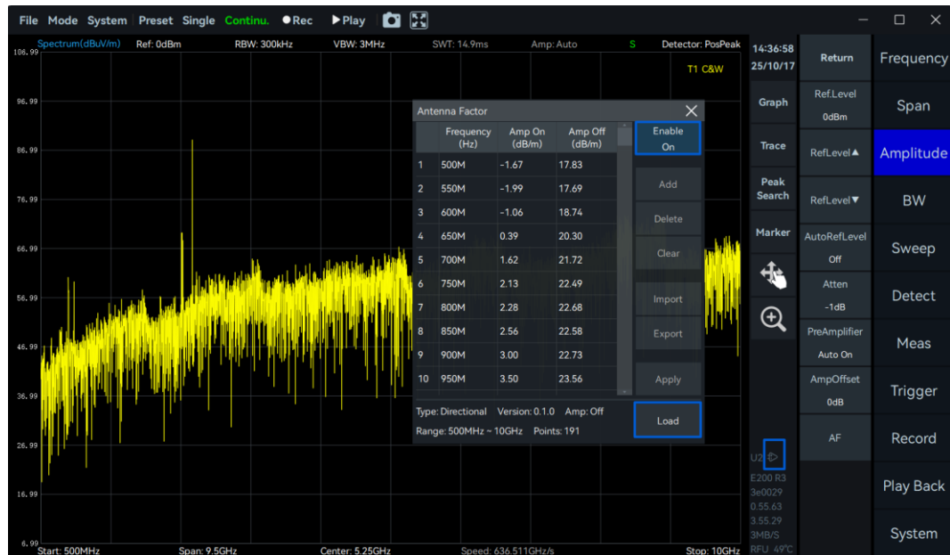
Figure 25 With HDA-100: automatic loading of antenna factors
