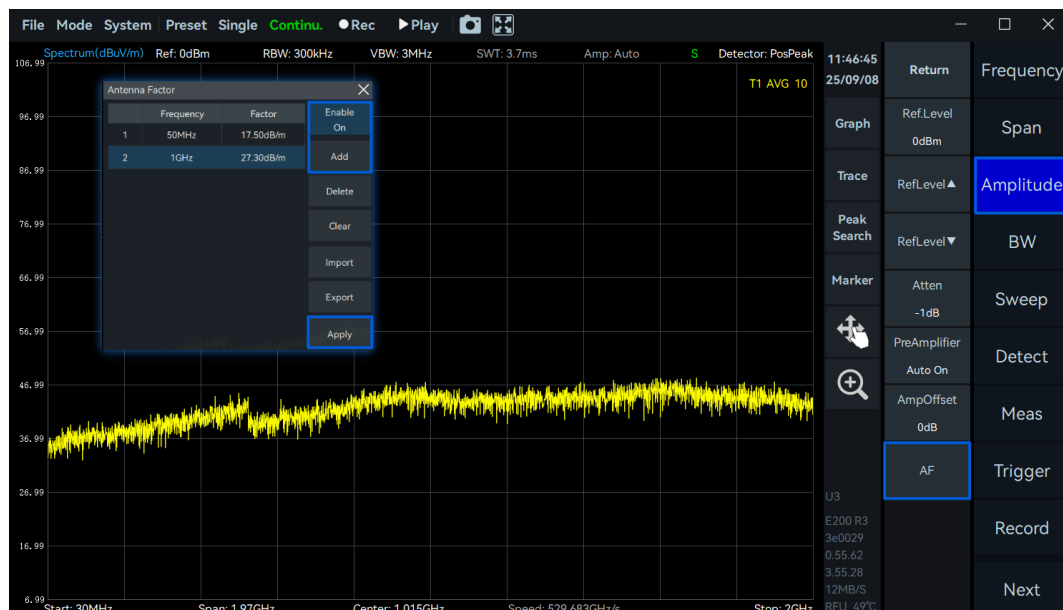
Figure 24 Antenna Factor Configuration Example
