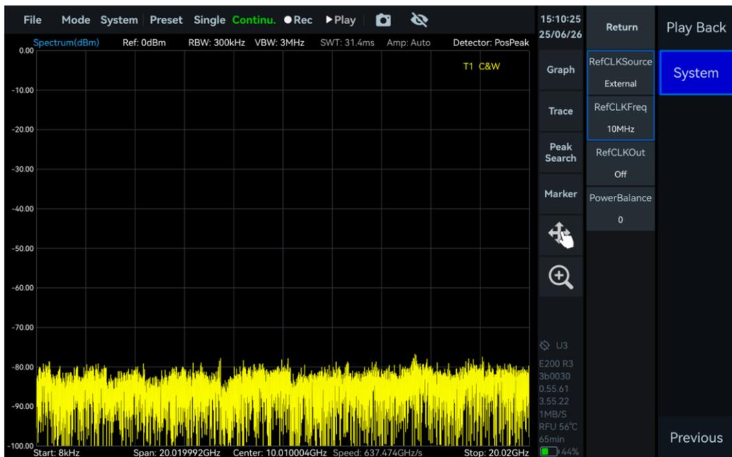
Figure 47 Use External 10MHz Reference Clock
