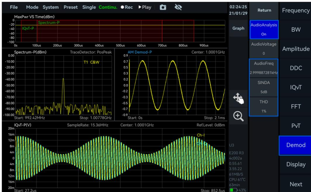
Figure 18 AM Demodulation Audio Analysis
