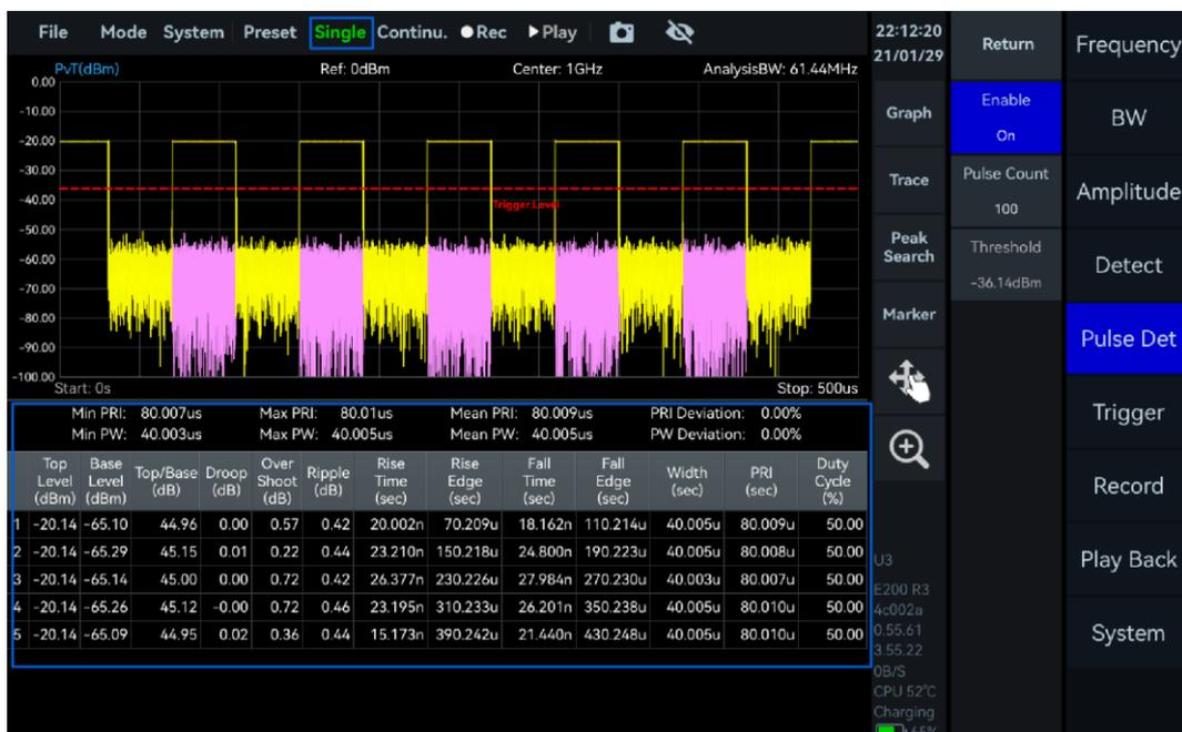
Figure 37 Result of Pulse Detection
