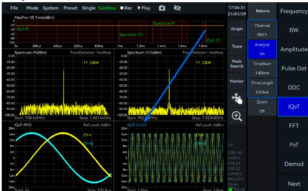
Figure 32 View Time-Domain Graph of IQ Substream under DDC
