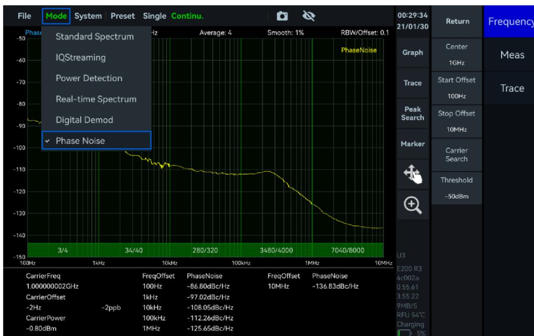
Figure 42 Enable Phase Noise Measurement
