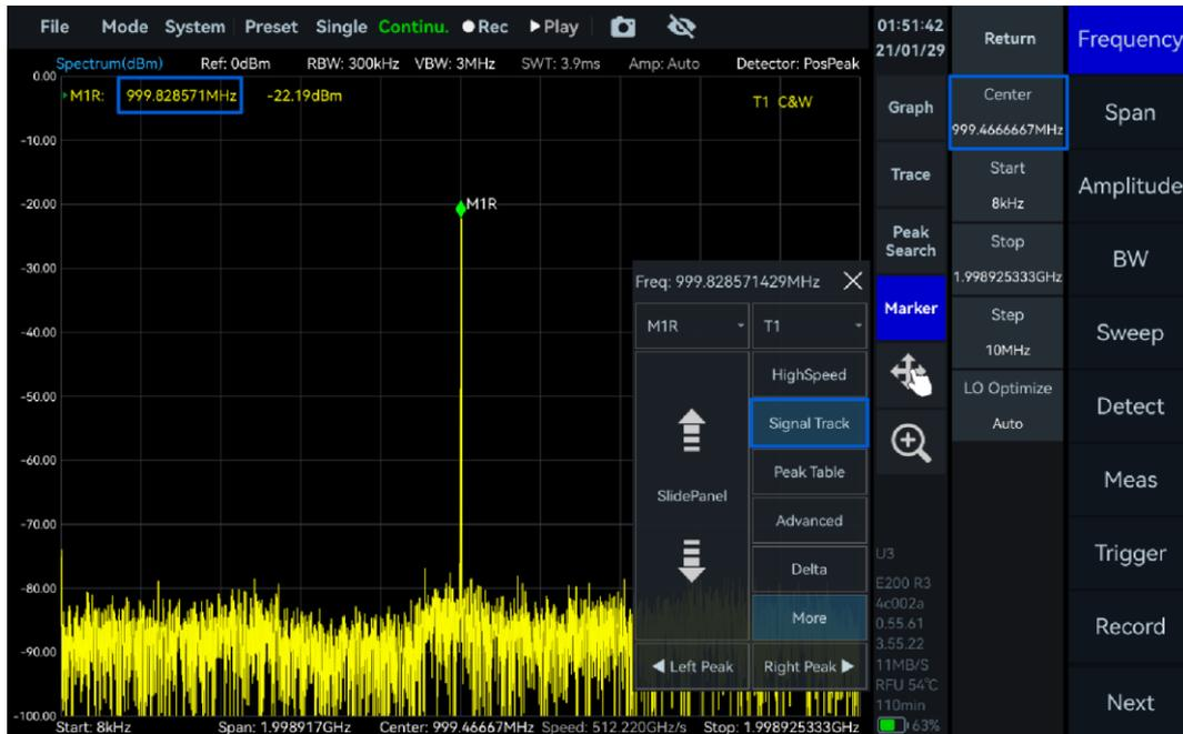
Figure 24 Frequency Tracking
