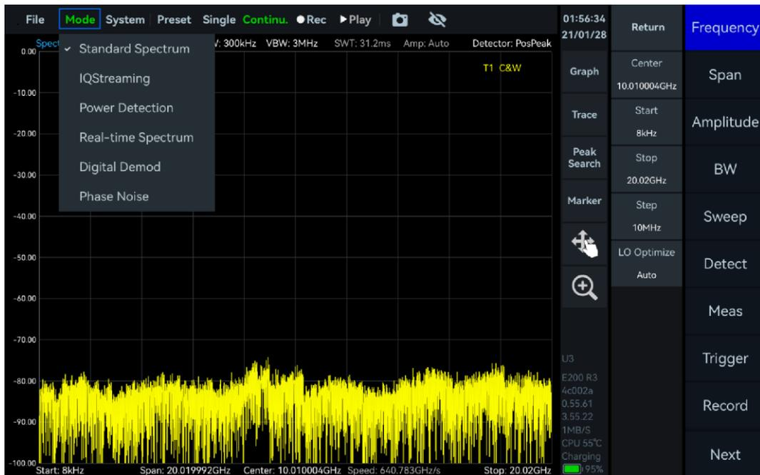
Figure 3 Working Mode Switch
