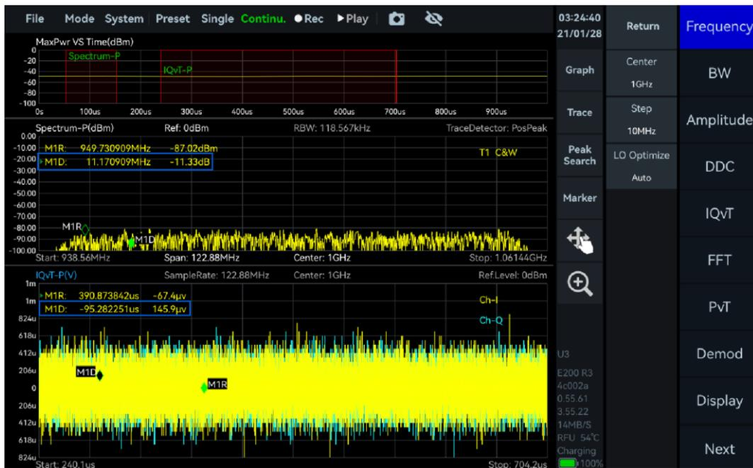
Figure 12 Enable Delta Marker
