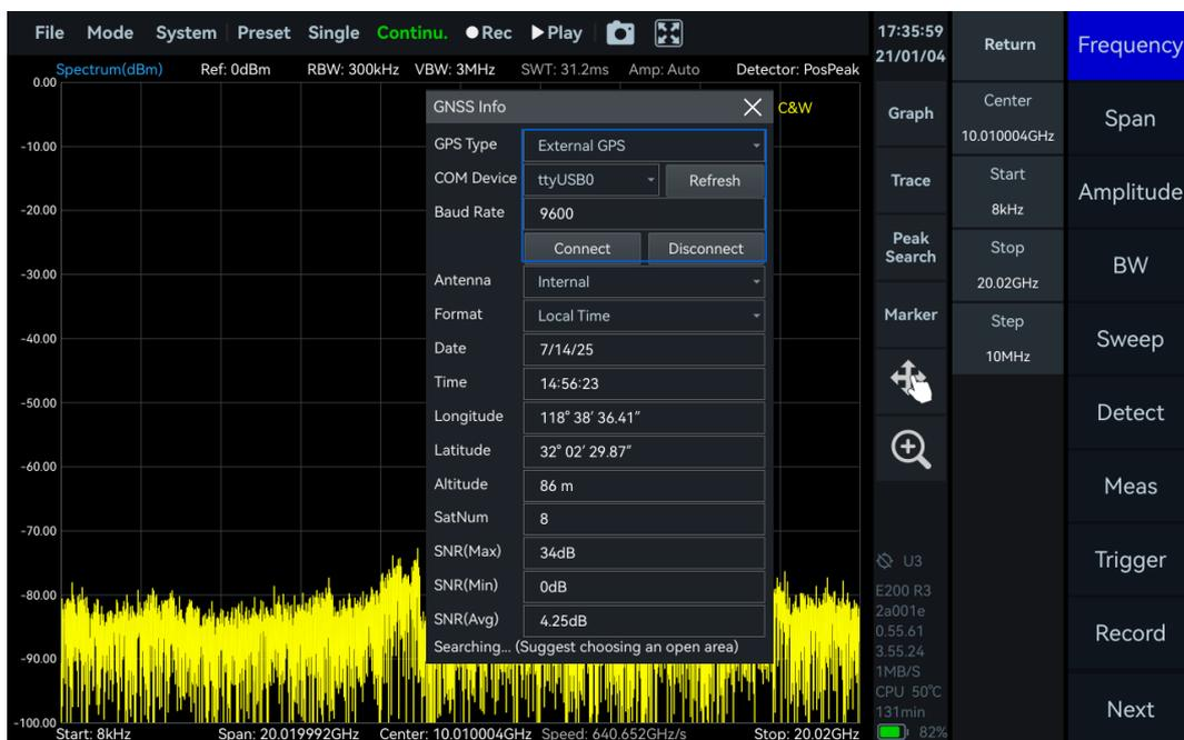
Figure 14 Connecting an external GNSS module
