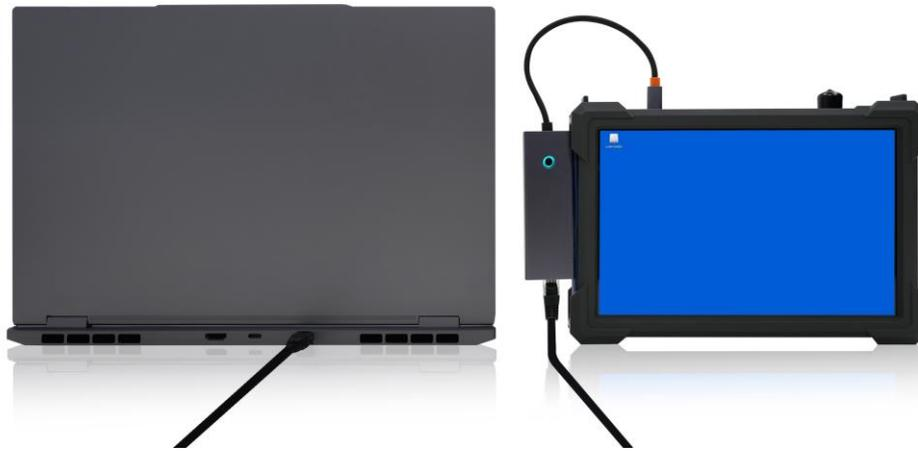
Figure 53 Remote Control of PX Instrument via Direct Ethernet Connection
