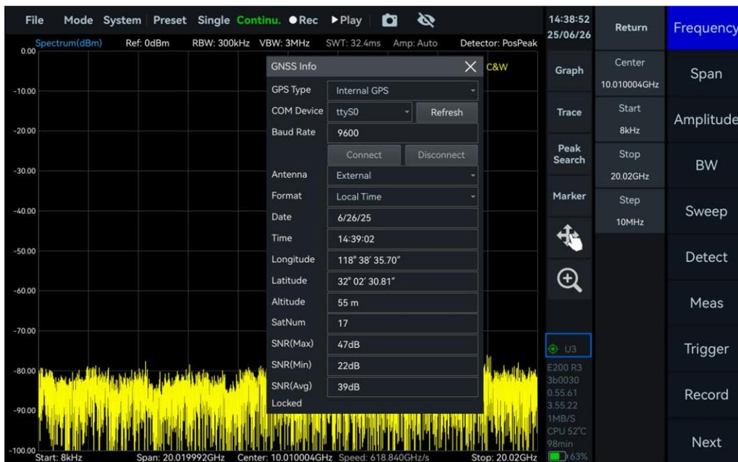
Figure 16 Locked GNSS external antenna
