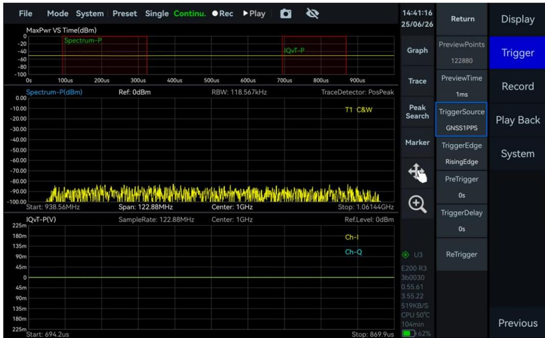
Figure 17 Triggered by GNSS 1 PPS
