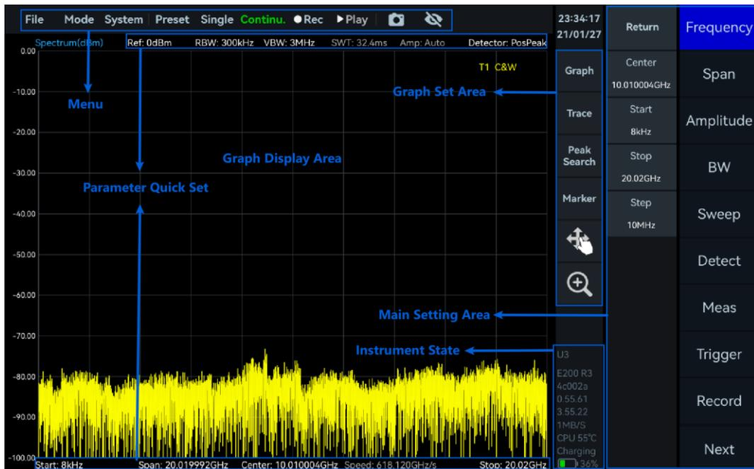
Figure 2 Application Software UI Layout
