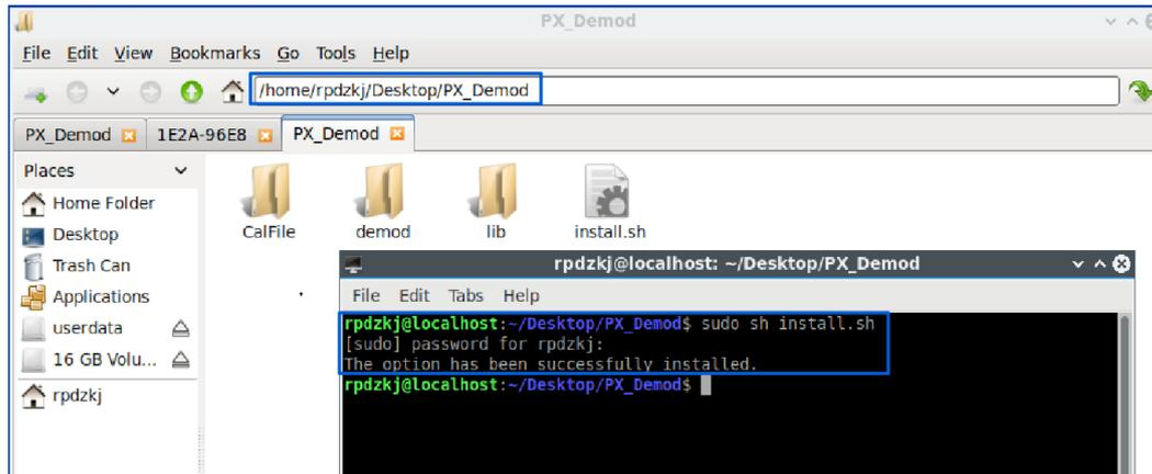
Figure 35 Install License of Pulse Detection Option
