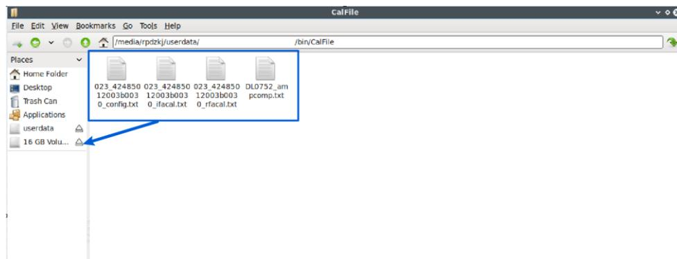
Figure 58 Obtain Instrument Calibration File
