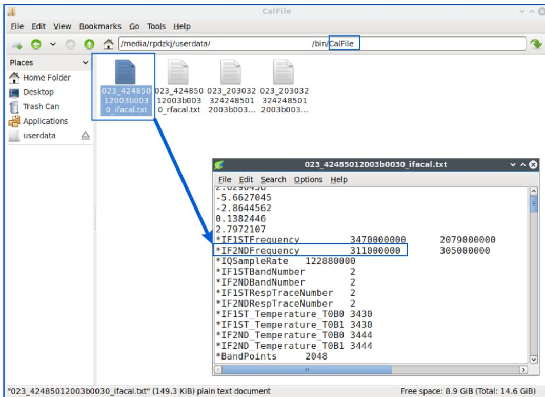
Figure 45 Check Center Frequency of IF Output
