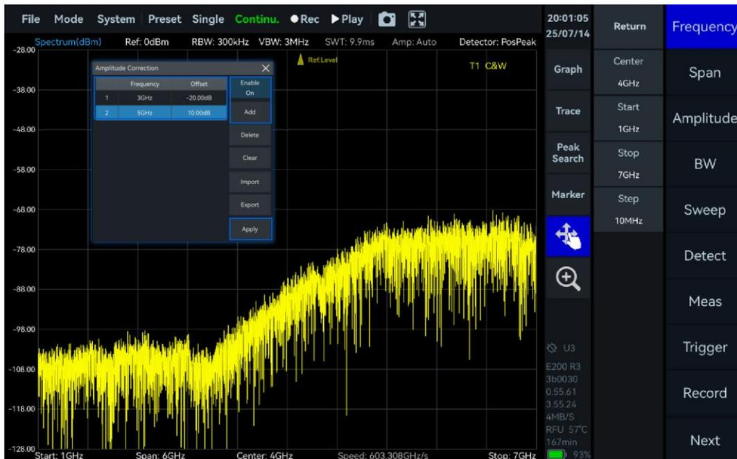
Figure 11 Amplitude correction application
