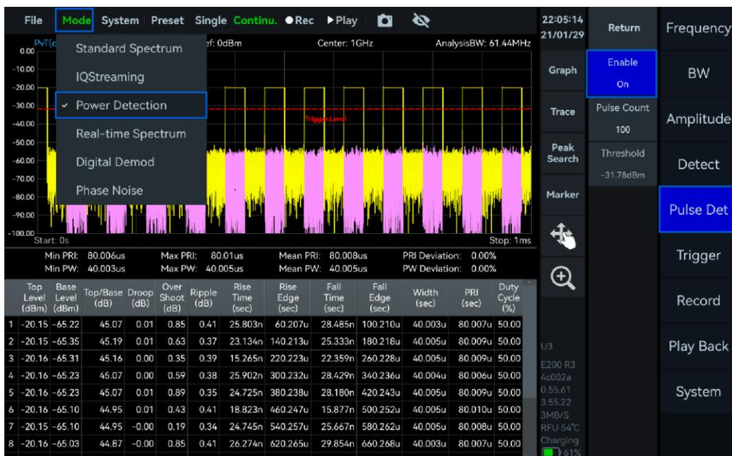
Figure 36 Enable Pulse Detection Measurement
