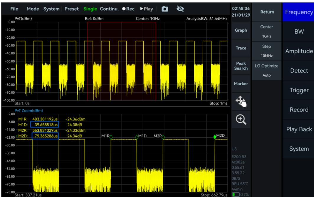
Figure 34 Measure Pulse Signal Period and Width
