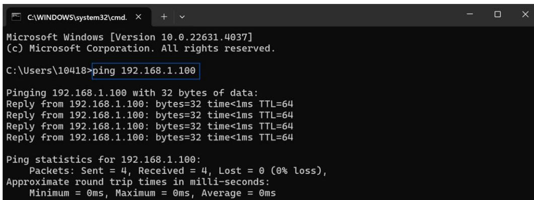
Figure 50 Test Network Connection of Instrument (ping command)
