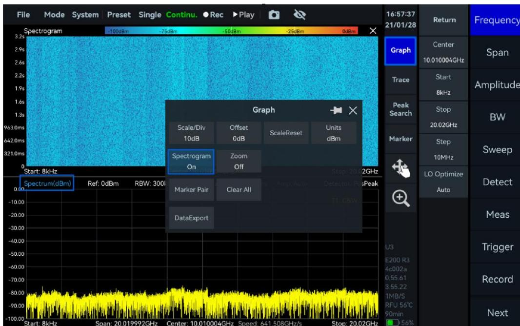
Figure 5 Enable Spectrogram
