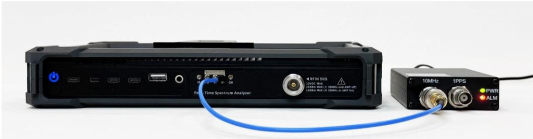
Figure 46 10MHz Reference Clock Input
