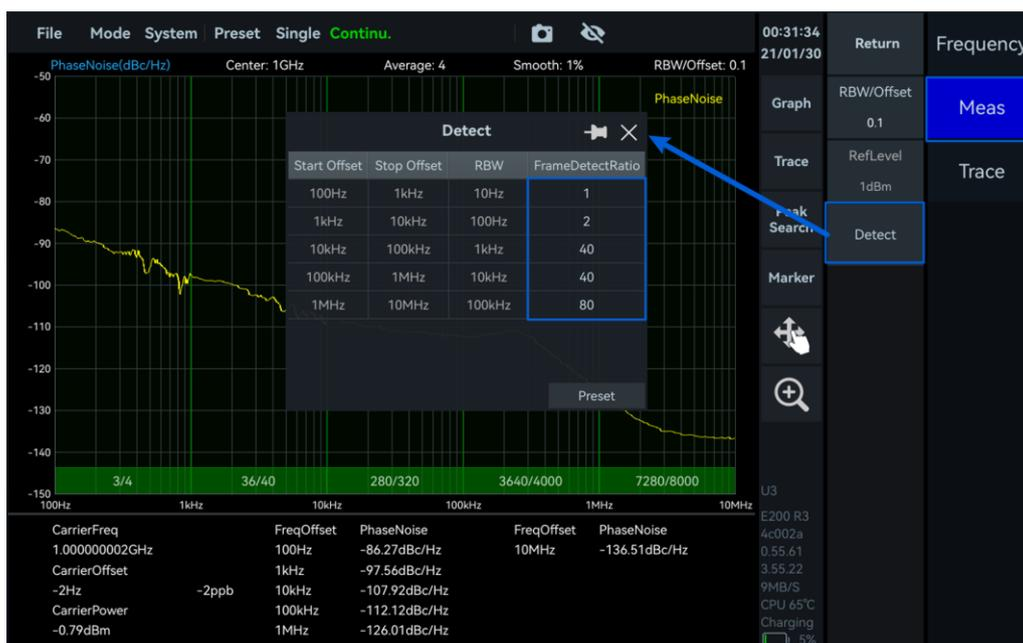
Figure 43 Settings of Pulse Signal Detection
