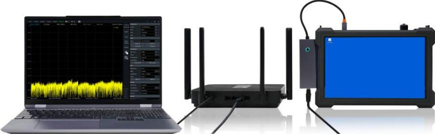
Figure 59 Remote Control PX Instrument via LAN
