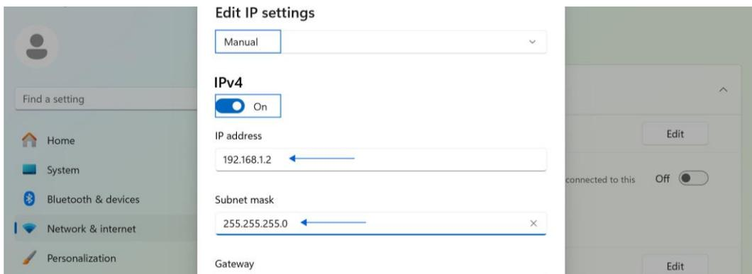
Figure 49 IP Address and Subnet Mask
