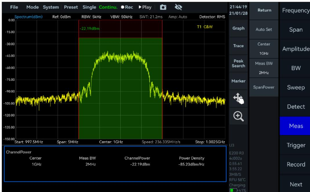
Figure 18 Measure Channel Power
