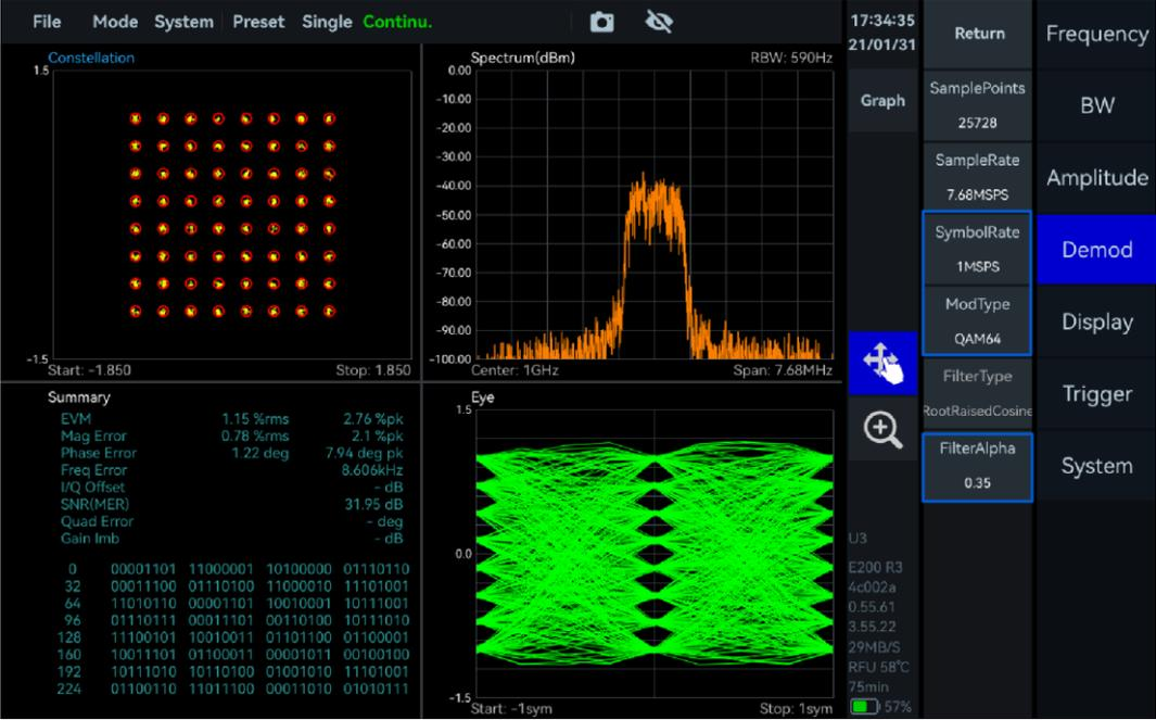
Figure 40 64QAM Demodulation
