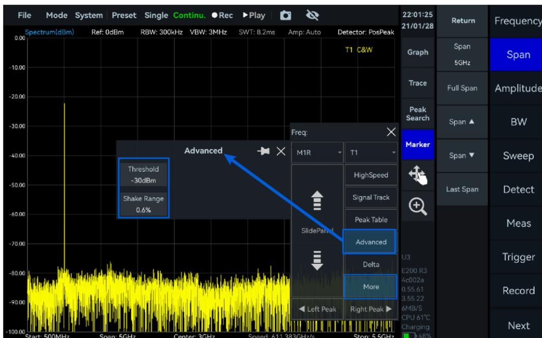
Figure 23 Set Peak Threshold and Jitter Range
