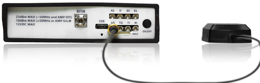
Figure 6: NX Series Instrument External Antenna Connection Diagram
