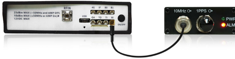
Figure 8 External Reference Clock Connection Diagram for NXE/NXN-400
