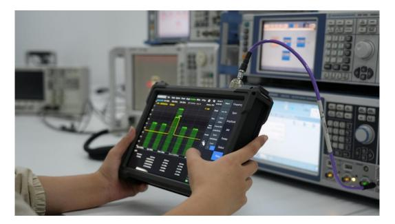
**Portability and Battery Life:** Field and on-site testing often take place away from the office, so instrument weight and battery life directly impact work efficiency. Choose an HSA with low weight and a battery that can support continuous use for at least a full workday (e.g., 3-6 hours). A replaceable battery design or extra power bank support is also a significant advantage.
